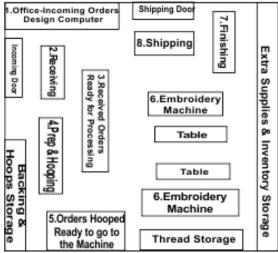
Now here is a drawing of a basic layout for a small shop that has two, two-head embroidery machines. This was actually created for a small shop that had a retail front end with a separate room for their embroidering. This was a large 16 by 16 foot room in the back of the store. The best physical layout of your shop will determine how you will be able to place your machines for the best possible production.
